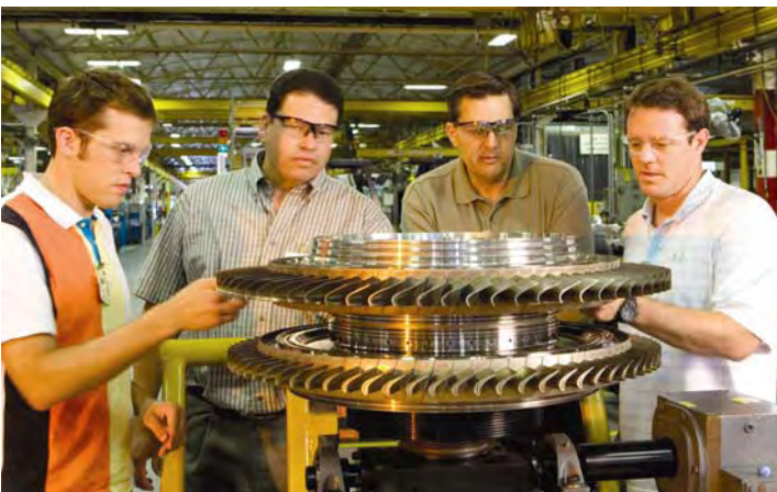
Figure 13. Gas Producer Turbine
