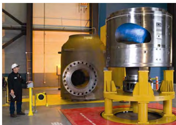
Figure 19. Gas Compressor Assembly
