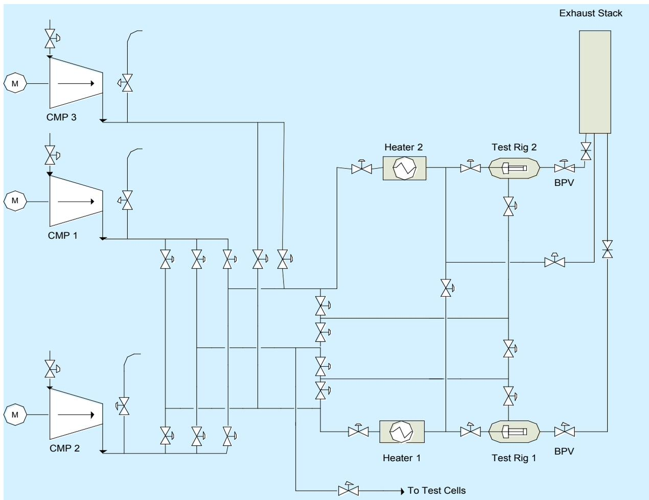
**Figure 3:** Diagram of HPAD system.
