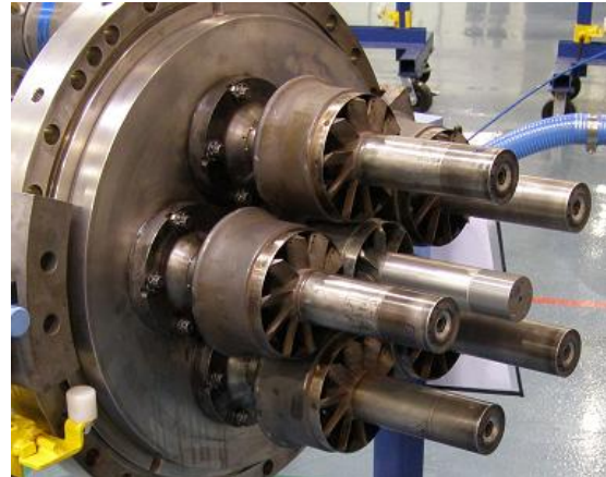
Figure 3: End Cover assembly prior to repair [4]
