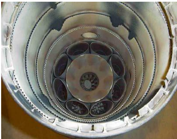
Figure 4: DLE Combustor showing damage due to flashback [2]
