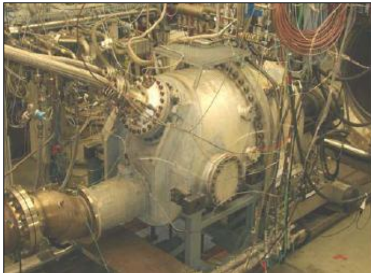
Figure 3: Single Combustor, Full Pressure Test Rig
