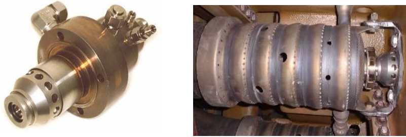
Figure 4: Conventional or Diffusion flame combustion hardware
