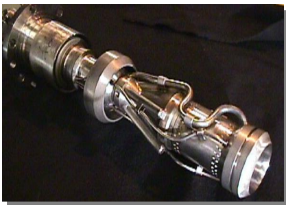
Figure 10: Annular Combustor with 3 rd generation DLE burner
