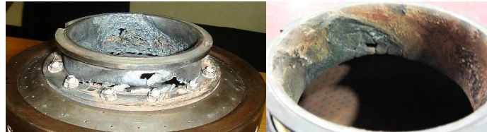
Figure 1: DLE Pre-chamber damage resulting from hydrocarbon carry over and oxidation
